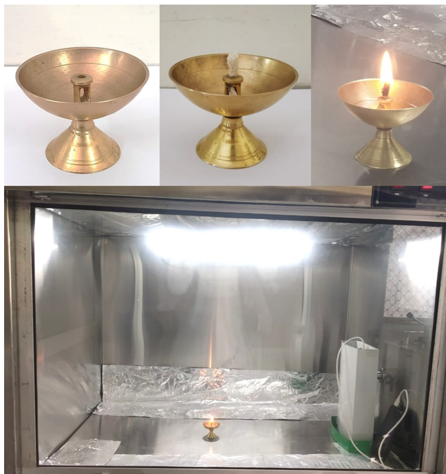
Figure 1: Experimental Setup. Top panel of the image shows the metal lamp (left), metal lamp containing muslin cloth wick (middle), and bottom image shows bio-safety cabinet containing oil lamp and gas analyzer.
